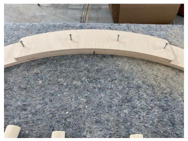
After the other side of the arch is assembled, attach with the connector facing outward. Then attach with the dowels that are already on the other side.
