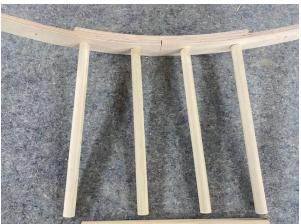
Then attach the rest of the arch dowels loosely to the remaining holes with bolts in them.
