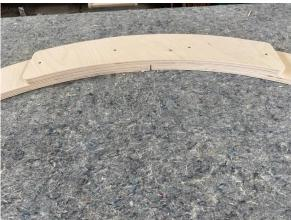
After the connector covers the arch spilt, then insert bolts. After the bolts are inserted, flip the piece on its side and attach 4 arch dowels loosely.
