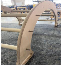
Once all your arch dowels are attached to both arch side pieces, then you are ready to tighten all the bolts securely.
