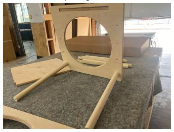
Then, attach the other side of the cube to the dowels with the bolts(very loosely).
